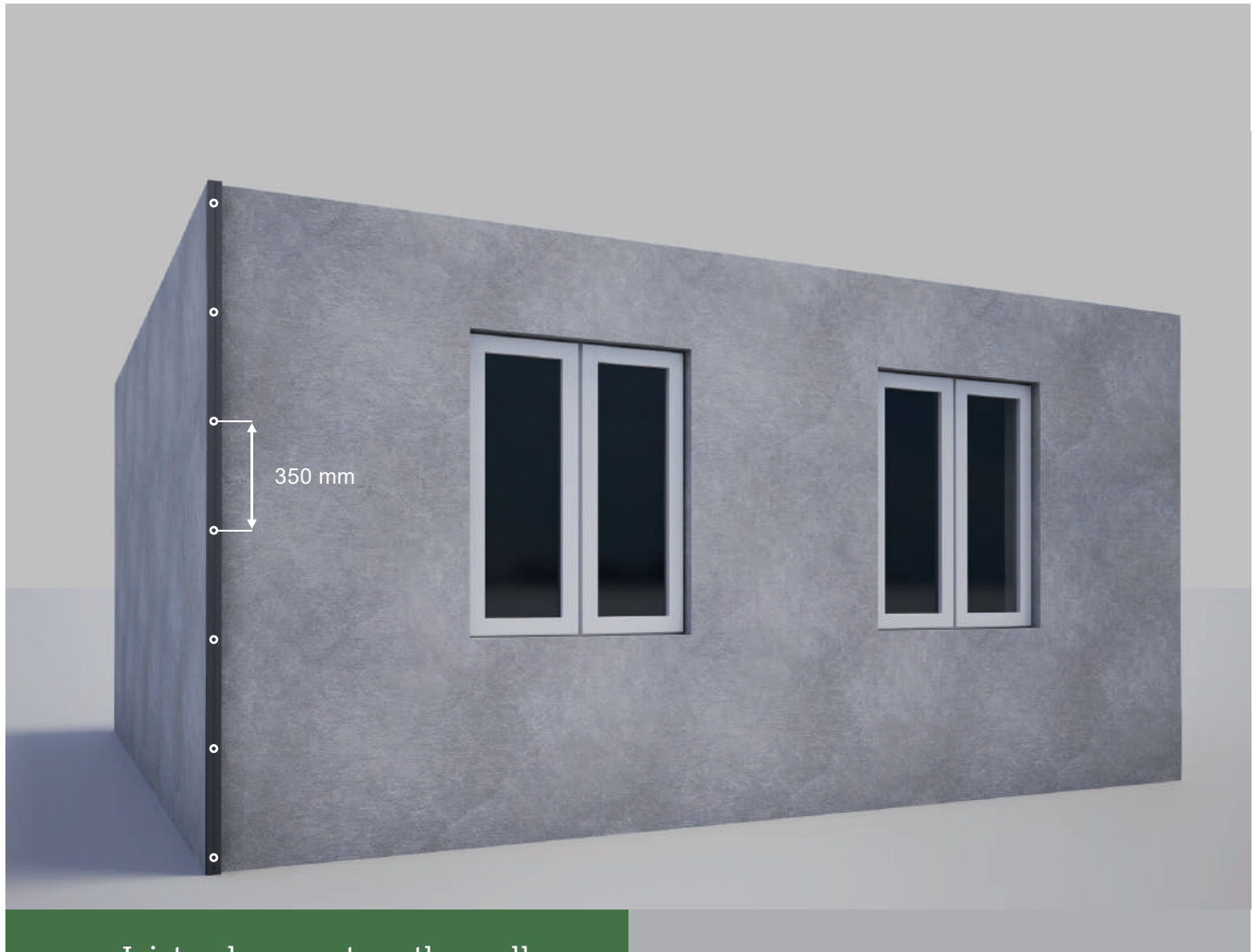
Joists placement on the wall
