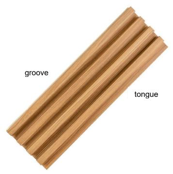
Place the clips evenly (approx. every 50 cm) on the protruding part on the groove side. Screw it to the wall. Then insert another board into the groove (tongue side) and mount it with the clips. Repeat the process with the consecutive boards.
